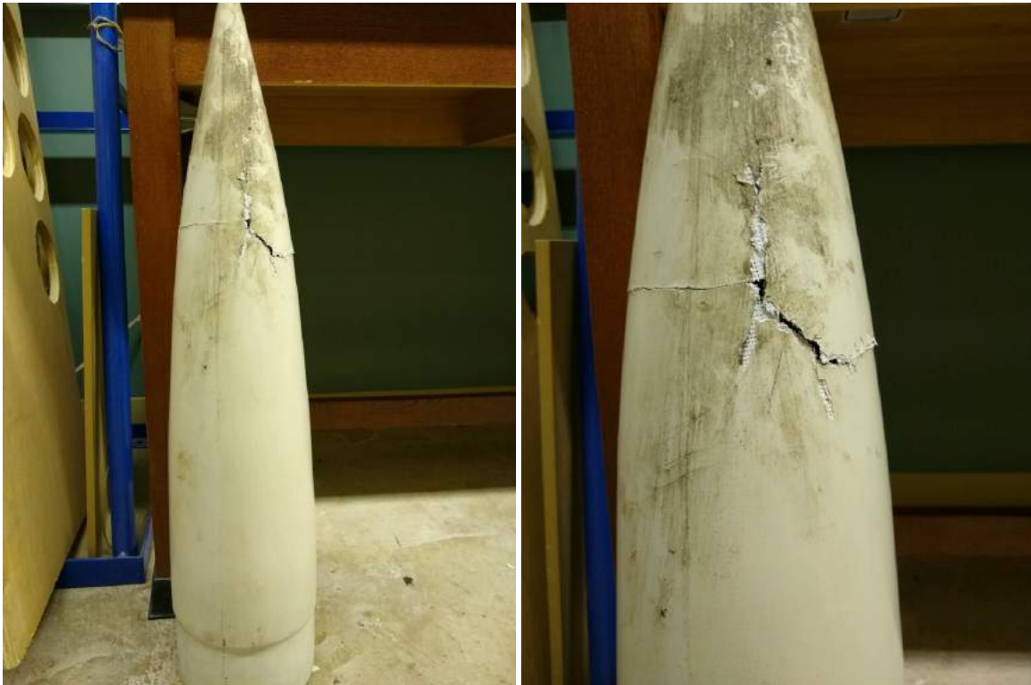
Figure 6: Nose Cone Damage
