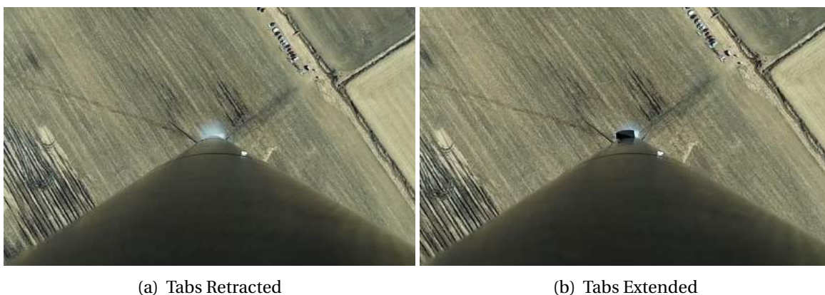
Figure 19: ABS tab actuation during flight
