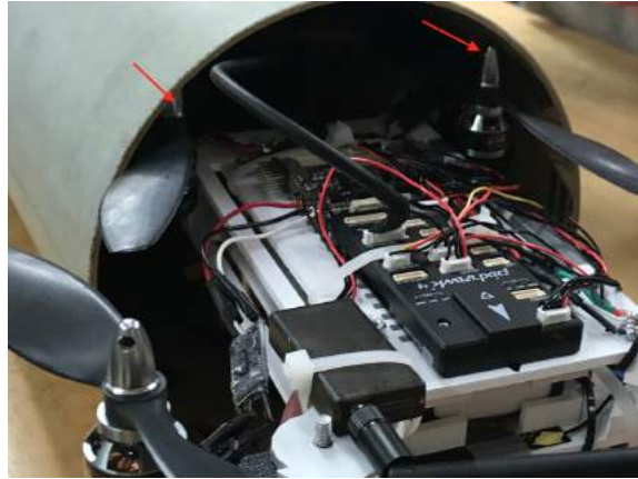
Figure 15: Red arrows highlight the points where the drone touches the inner wall of the body tube.
