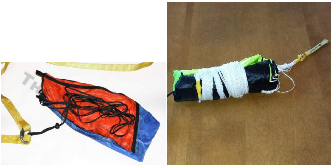
Figure 9: As launched packing (left) vs. the new packing method (right) Photos courtesy of Rocketman Enterprises and Fruity Chutes Inc.
