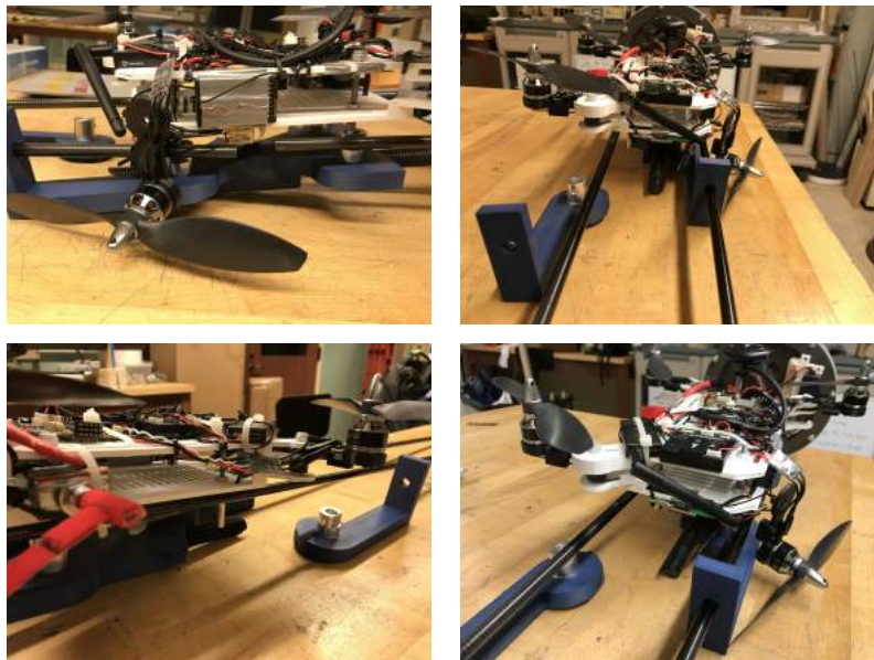
Figure 14: Broken hardware for this year's scoring payload.
