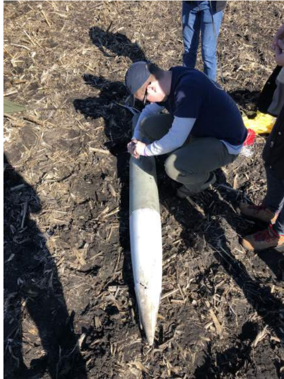
Figure 11: Nose cone still securely attached.
