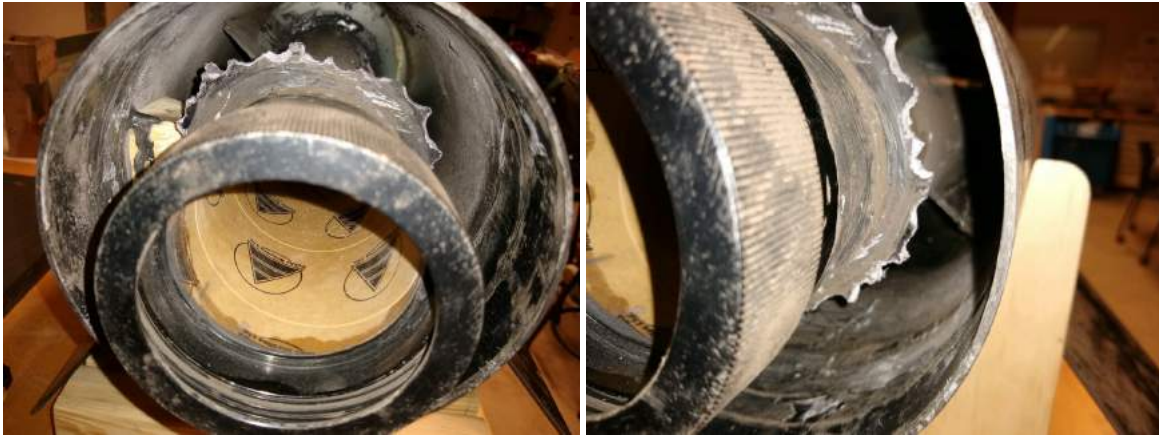
Figure 4: Centering Ring post-removal
